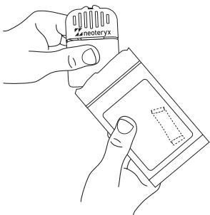
2. Open the device by pulling tabs on device apart from each other until the two flaps are folded downwards. **NOTE:** Do NOT remove sampler tips from sampler bodies. Do NOT remove sampler bodies from device.
