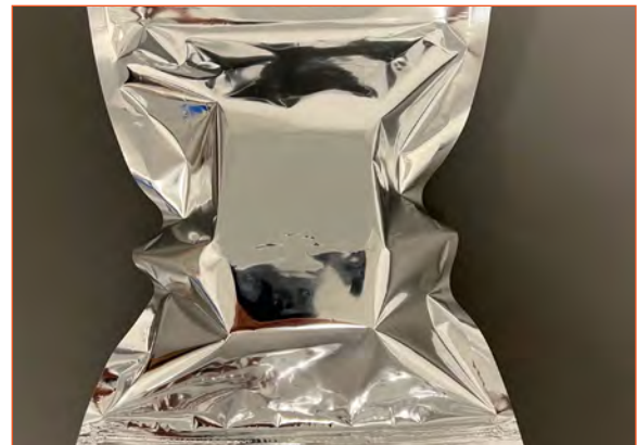
Sealed 8"x10" storage bags with fully loaded autorack and 96-well plate Filled storage bag dimensions are approximately 8" x 10" x 3.5" (W x L x H).
