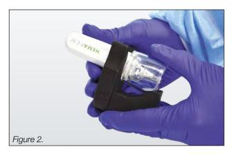
Gently push hemaPEN into the opening tool until the hemaPEN engages the V notch of the cradle. Inspect and ensure that the cutting blade has engaged the main body (Figure 3).
