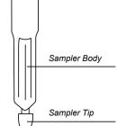
entire sampler tip turns red indicating a volumetric sample (10, 20, or 30 µL depending on the device being used) has been collected. This process is repeated for each sampler tip in the device.
