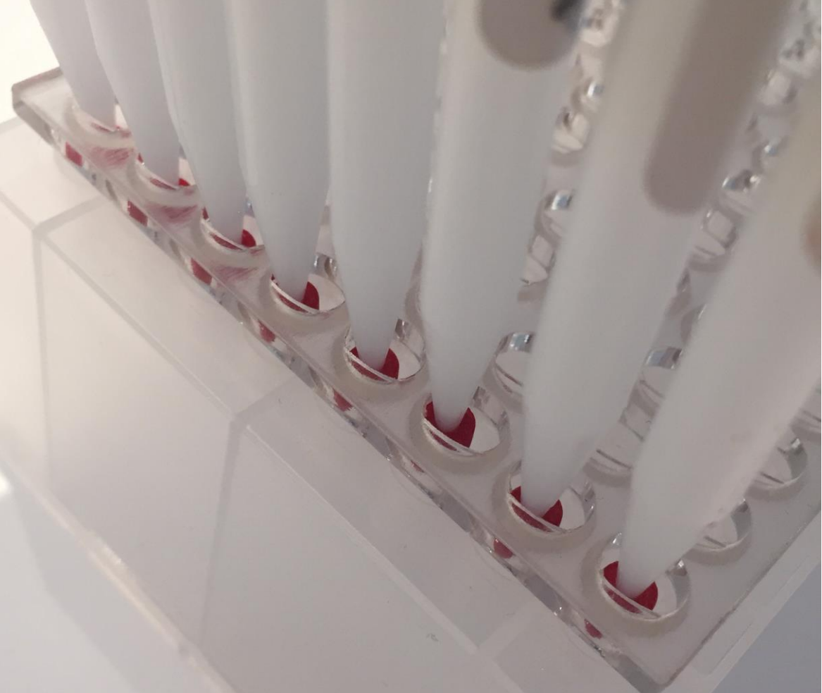
Figure 1: Picture displaying the use of the Mitra tip extraction prototype to remove the whole blood sample tips from the Mitra and drop into a 96-well plate containing the 200 uL ethyl acetate:methanol (50:50, v/v) for extraction
