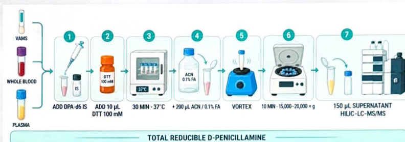
Figure 2. Sample-preparation workflow for the LC-MS/MS determination of total reducible D-penicillamine in VAMS, whole blood and plasma. D-penicillamine-d 6 was added as the internal standard, followed by reduction with dithiothreitol for 30 min at 37°C. Proteins were precipitated with acidified acetonitrile, and the samples were vortex-mixed and centrifuged. The clear supernatant was transferred to an autosampler vial and analysed by HILIC-LC-MS/MS.
