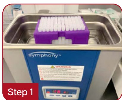
Step 1 Sonicate collection plate and 96-Autorack assembly for 15 minutes and/or
