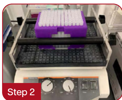
Step 2 Shake collection plate and 96-Autorack assembly on Vibramax 100 (Heidolph) for 1 hour @ 1200 rpm.
