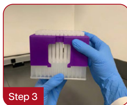
Step 3 Remove 96-Autorack containing Mitra devices from the collection plate and discard.
