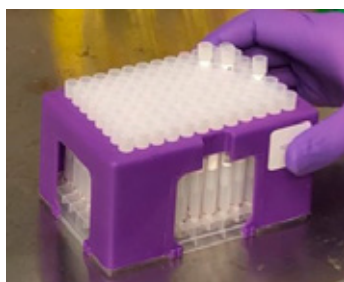
Figure 10. Lift the rack of 96 Mitra devices off its protective high wall microplate and place the rack of devices over the microplate. Some devices may not immediately drop into the well. Touch these gently and they will drop into place, then push the rack of device so it is flush with the bench surface.
